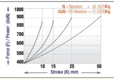
**Pressure Increse:** During operation, the piston of the gas spring inserts into the body and the volume of the gas inside gradually decreases. As a result, the pressure increase can be seen as the multiplication factor in the gas spring diagram. The spring force can be easily calculated by multiplying the initial force and the pressure increase factor.
