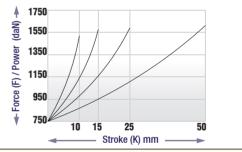
Adjusting filling pressure: It can be adjusted according to the spring force and determined by using spring diagram in advance. Spring forces according to spring diagram: The stroke increase / spring force replacement, pressure increase factor and replacements are considered, however you should take into consideration external effects.
